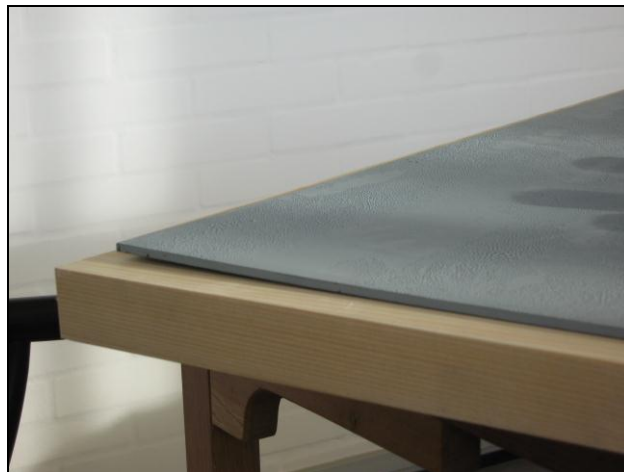
Figure 1.5. The corner of the double spanning plate lifts up at the corner.
